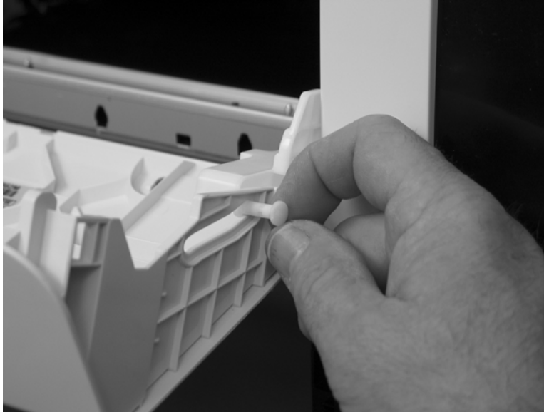
Figure 1-53 Remove the front door and front-lower cover (6 of 8)
