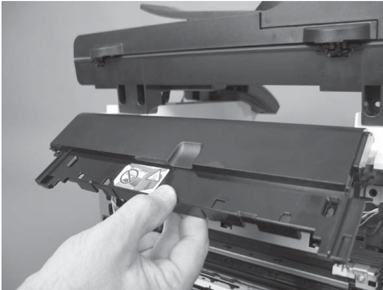
Figure 1-42 Remove the rear-upper cover (4 of 4)
