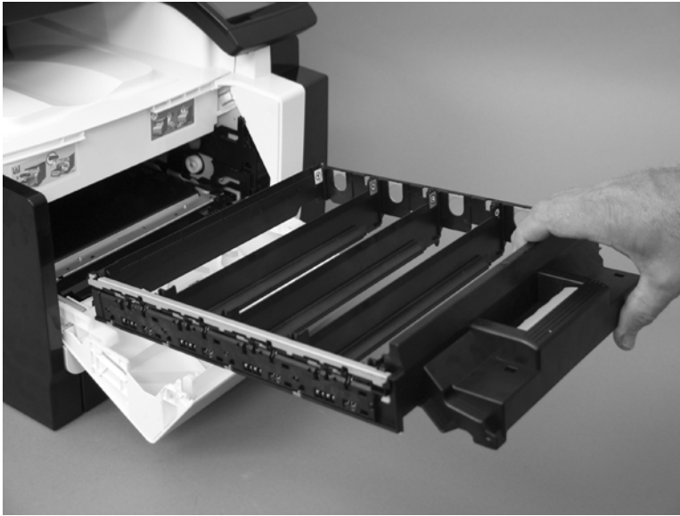
Figure 1-13 Remove the print-cartridge drawer (5 of 5)
