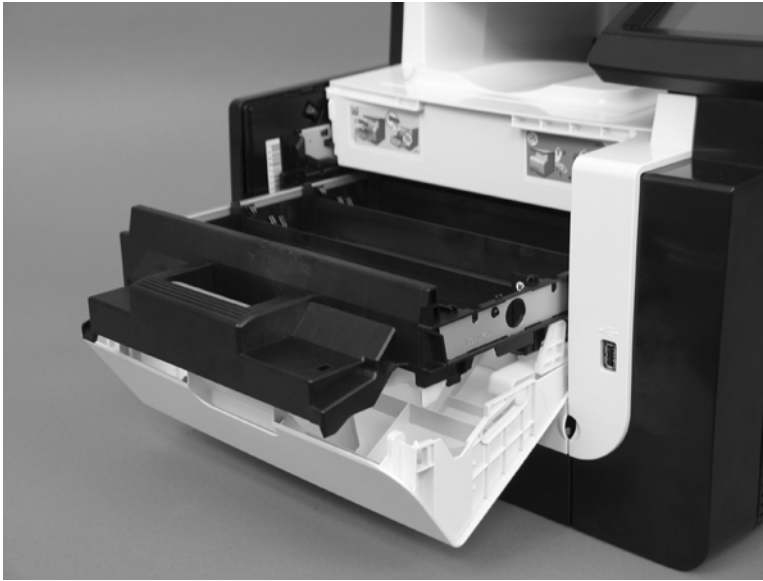
Figure 1-9 Remove the print-cartridge drawer (1 of 5)
