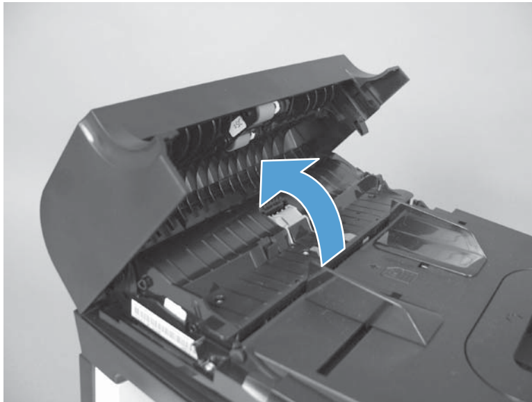
Figure 1-128 Remove the document feeder input tray (1 of 2)
