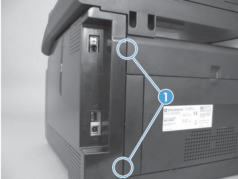
Figure 1-16 Remove the right cover (3 of 5)
