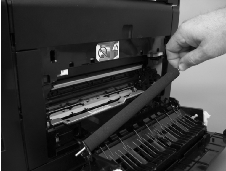
Figure 1-8 Remove the transfer roller (3 of 3)
