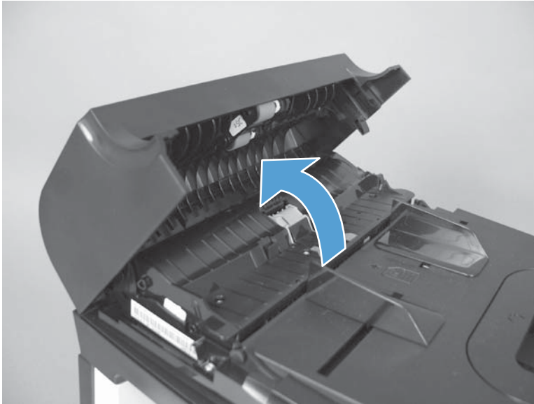
Figure 1-130 Remove the document feeder cover (1 of 3)
