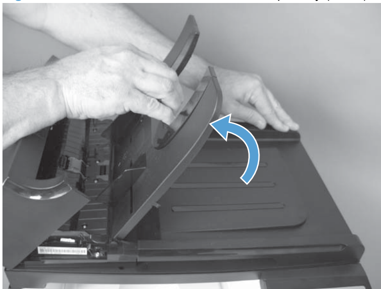
Figure 1-129 Remove the document feeder input tray (2 of 2)
