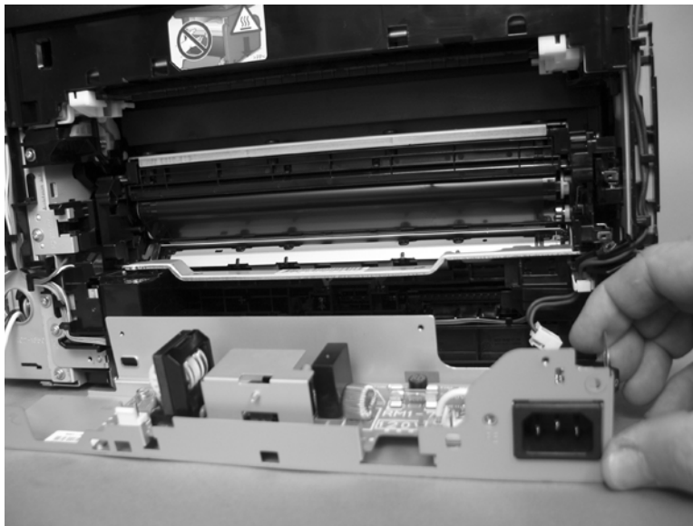
Figure 1-116 Remove the power supply (fuser; 5 of 5)
