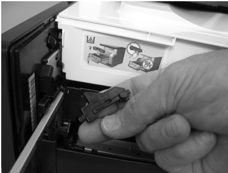
Figure 1-12 Remove the print-cartridge drawer (4 of 5)
