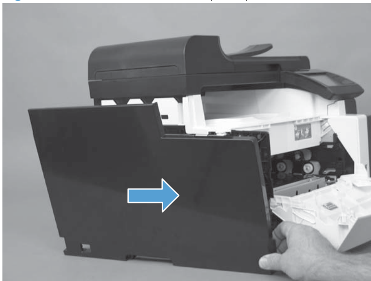
Figure 1-33 Remove the left cover (6 of 6)
