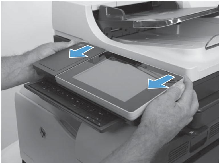
8. Slightly lift up the control-panel assembly to access the FFC-keyboard connector.
