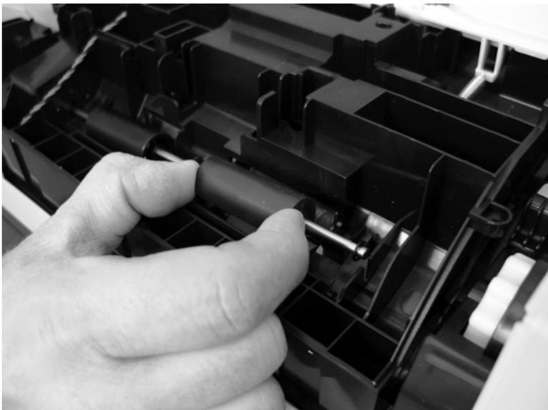
4. Open the document feeder jam access cover. Release one hinge.
