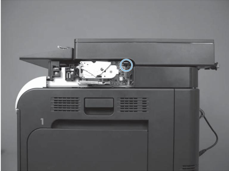
3. Remove one screw on the left side of the scanner.
