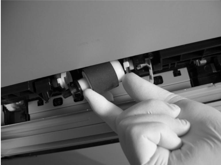
4. Remove the pickup roller.
