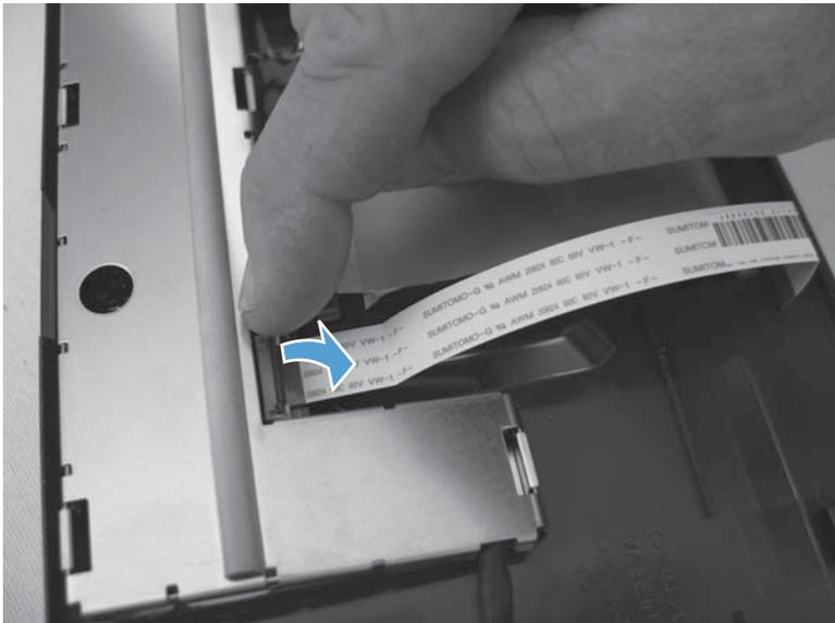
4. Slightly pull on the FFC to verify that it is securely fastened in the connector.
