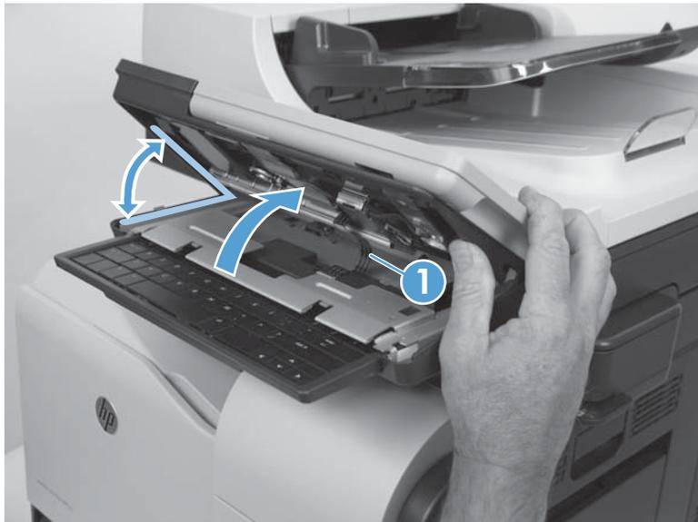
When removing the control panel, **do not** fully raise the control panel to access the FFC connector. Doing so causes strain damage to the FFC (callout 1).
