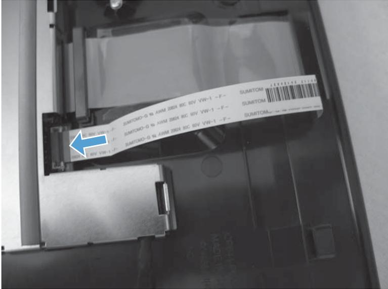
3. Use your finger to carefully close the connector retainer to lock the FFC in place.
