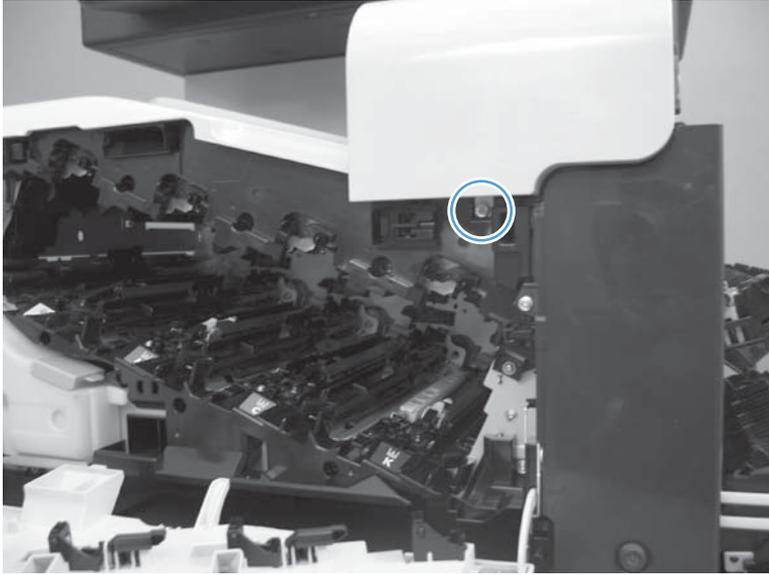
4. Lift the cover up, and then remove the front-upper cover.
