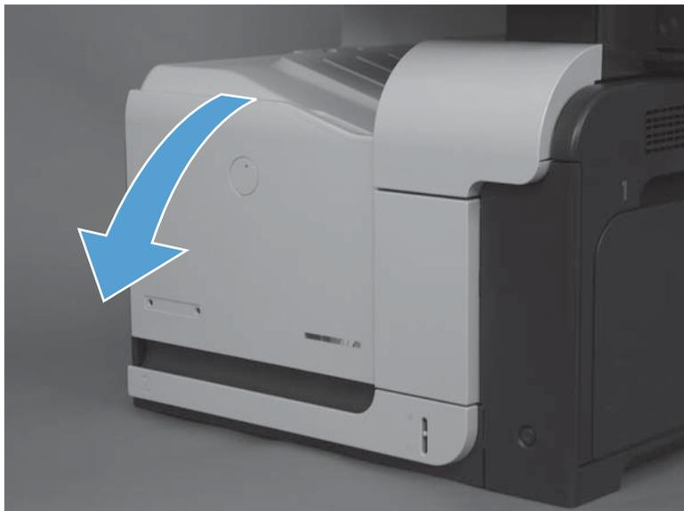
2. Remove two screws (callout 1), and then remove the front-door assembly.
