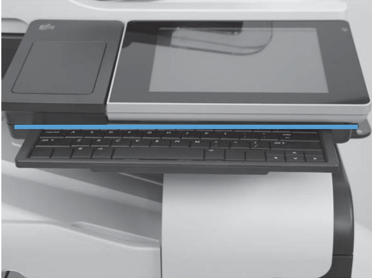
3. Lift the control-panel assembly to an upright position.
