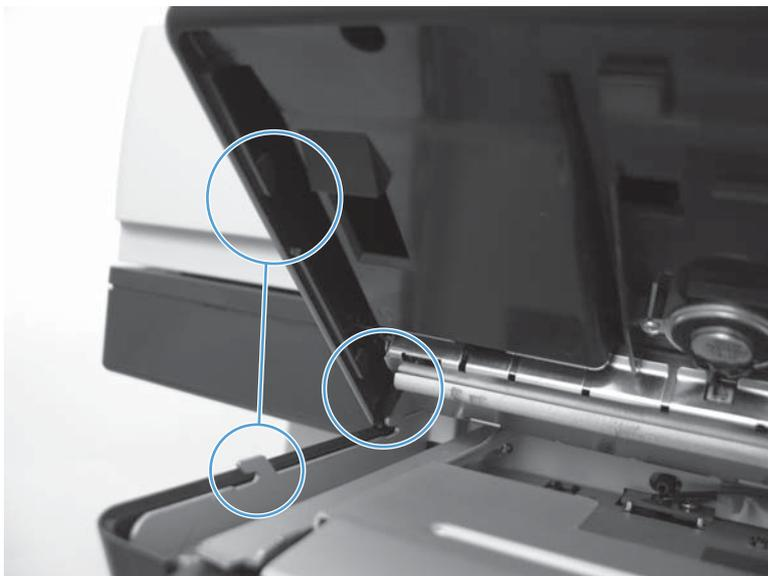
8. Reinstall the control-panel assembly on the product, and then push it up to engage the assembly with the chassis.
