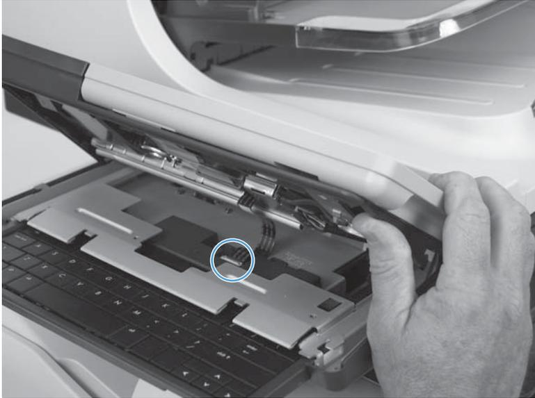
10. Carefully lift up on the connector retainer to release the FFC.
