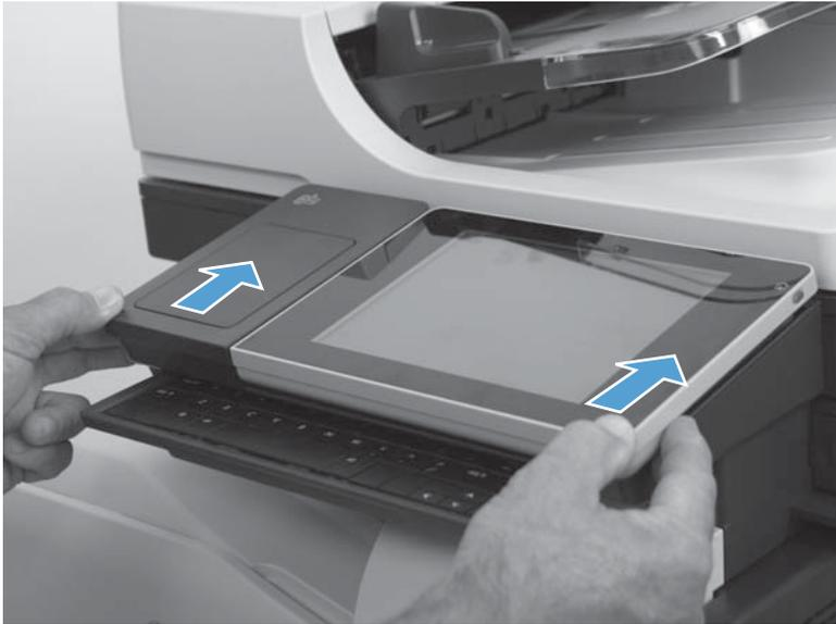
9. Carefully place the control-panel assembly in the raised position.
