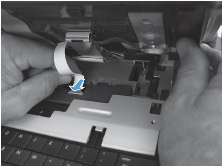
4. Use your finger to carefully close the connector retainer to lock the FFC in place.
