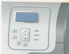
**EN** When prompted, select YES for NEW FUSER KIT. If the prompt does not appear, press Menu . Select CONFIGURE DEVICE > RESETS > RESET SUPPLIES > NEW FUSER KIT > YES.
