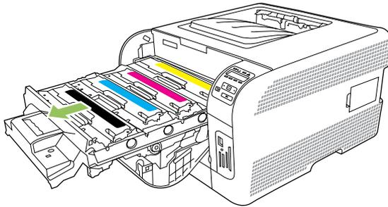
3. Grasp the handle on the old print cartridge and then pull the cartridge straight up to remove it.
