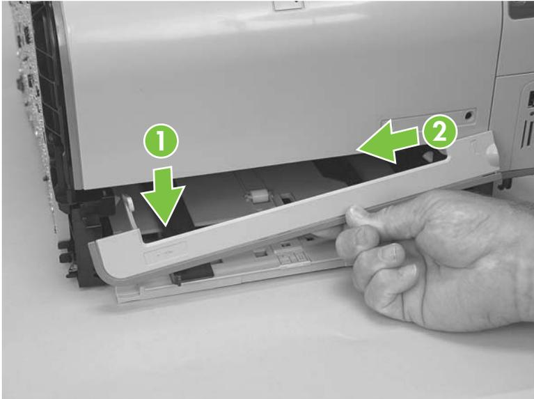
4. Open the front door, and then use a small flatblade screwdriver to release one tab (callout 1) on the left-side front-door cam.
