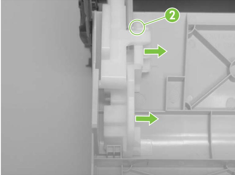
6. Carefully flex the edges of the door to release the right- and left-side door retainer arms.
