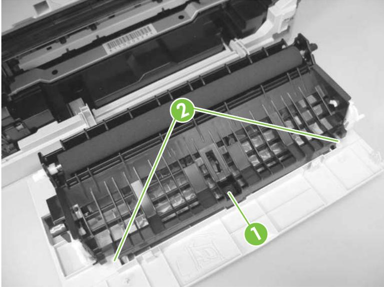
2. Remove the transfer roller assembly
