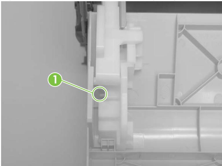
5. Slide the cam toward the center of the door to remove it. Repeat this step for the right-side front-door cam.
