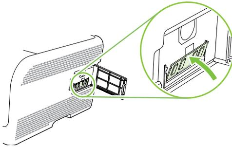
6. Push down on the DIMM until both latches engage the DIMM. When the installation is correct, the metal contacts are not visible.
