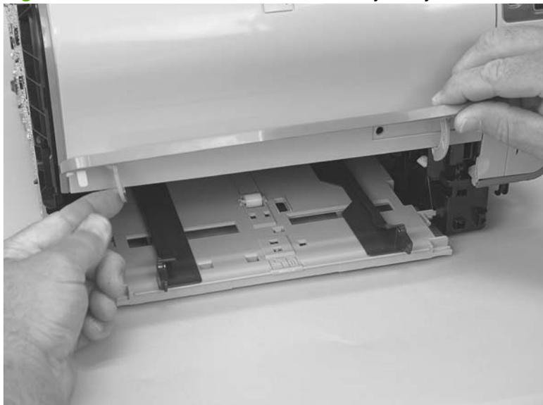
3. Lower the left side of the door and then slide it to the left to release the right-side hinge. Remove the door.
