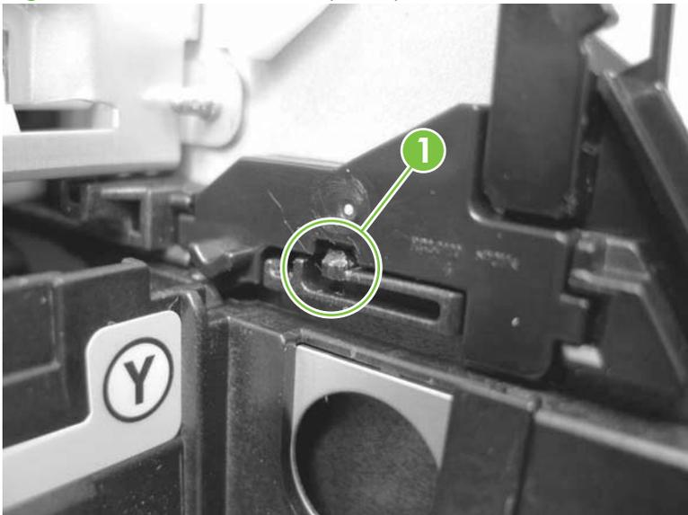
4. Rotate the cartridge-drawer retainer (callout 2) away from the chassis, and then remove it. Repeat the previous step and this step for the other cartridge-drawer retainer.
