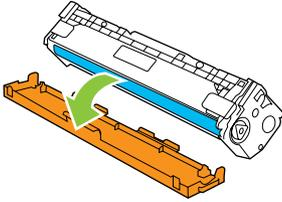
△ **CAUTION:** Do not touch the imaging drum on the bottom of the print cartridge. Fingerprints on the imaging drum can cause print-quality problems.
