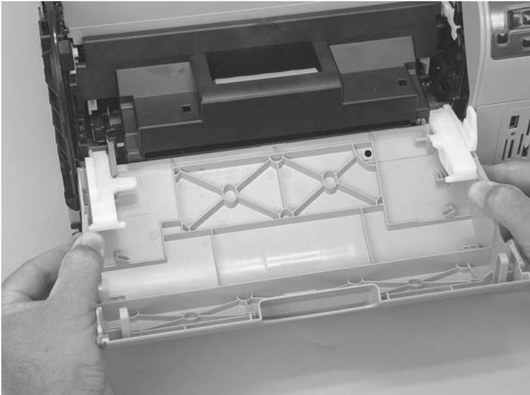
7. Lower the left side of the door, and then slide it to the left to release the right-side door hinge pin. Remove the door.
