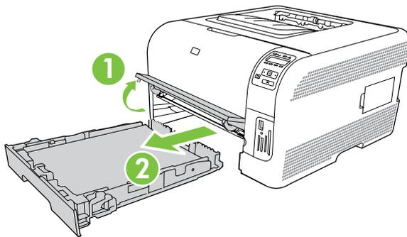
3. Push down on two tabs to release the Tray 1 panel (HP Color LaserJet CP1510 Series Printer).
