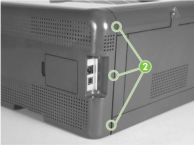
4. Rotate the bottom of the cover away from the product, and then slide it up to remove it.
