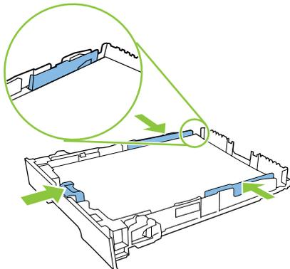
4. Push down on the paper to make sure that the paper stack is below the paper limit tabs on the side of the tray.
