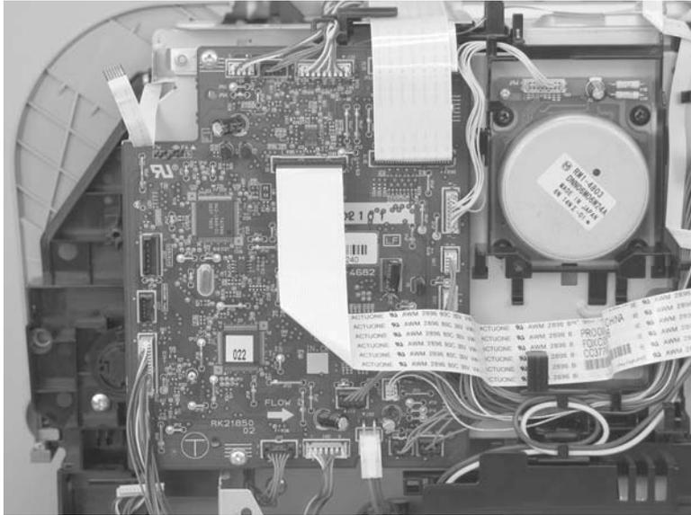
4. Remove four screws (callout 3), and then remove the DC controller PCA.
