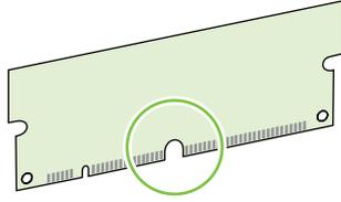
5. Holding the DIMM by the edges, align the notch on the DIMM with the bar in the DIMM slot at an angle.
