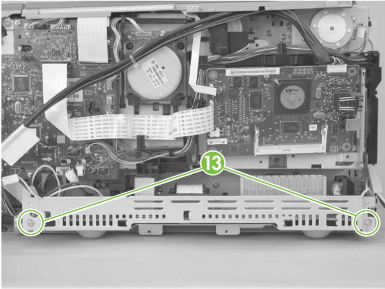
10. Pull the power supply away from the chassis (it will not come completely out).
