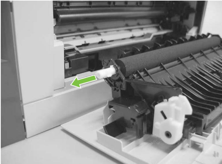
4. Slide the roller to one side to disengage the roller shaft from the mounting bracket, and then remove the transfer roller.
