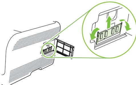
4. Remove the new DIMM from the antistatic package, and then locate the alignment notch on the bottom edge of the DIMM.
