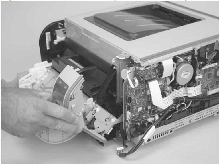
6. **HP Color LaserJet CP1510ni only:** Release one tab (callout 7), and then rotate the photo-card reader PCA toward the control-panel PCA to remove it.
