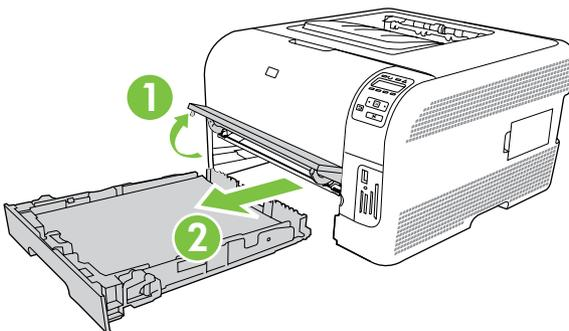
2. Remove the jammed sheet by pulling it straight out.
