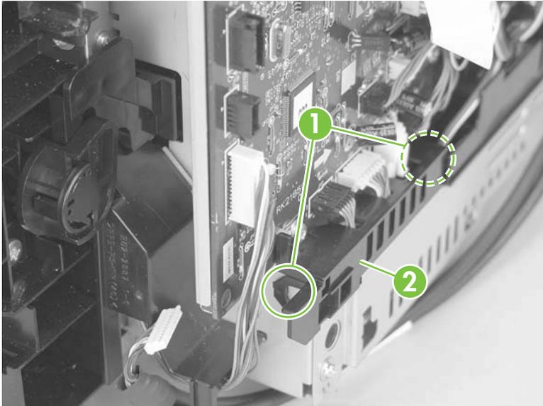
3. Disconnect all of the FFCs and wire-harness connectors from the DC controller PCA.
