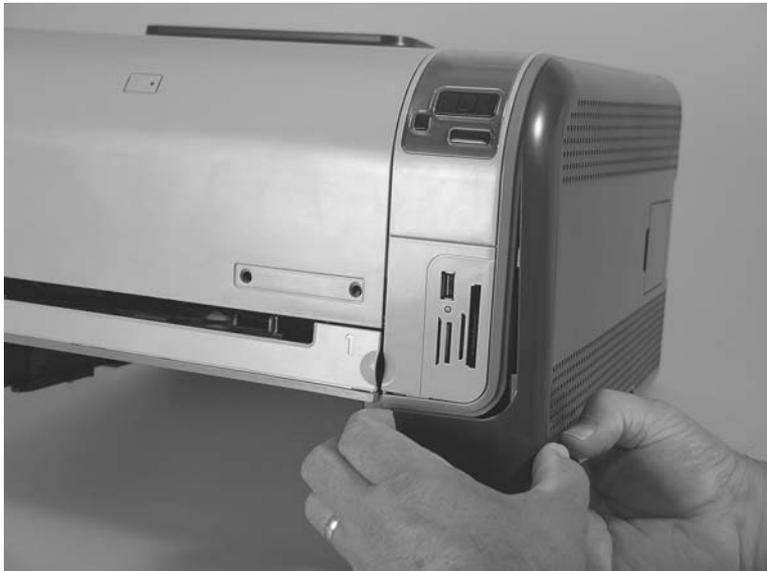
3. Use a small flatblade screwdriver to release three tabs (callout 2) at the back of the product.
