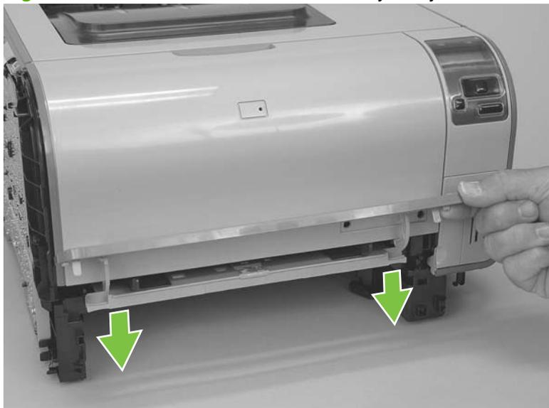
2. Carefully push the left-side Tray 1 or jam-access door hinge in toward the center of the door to release it from the hinge pin.
