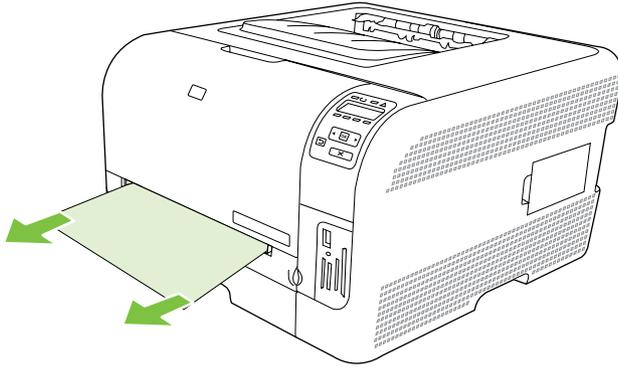
2. If you cannot see the jammed sheet, open the Tray 1 door (jam-access door) and pull out Tray 2.
