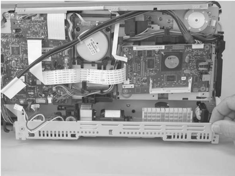
11. Rotate the end of the power supply near the control-panel module out and away from the product until it clears the chassis, and then slide the power supply toward the control-panel module to remove it.
