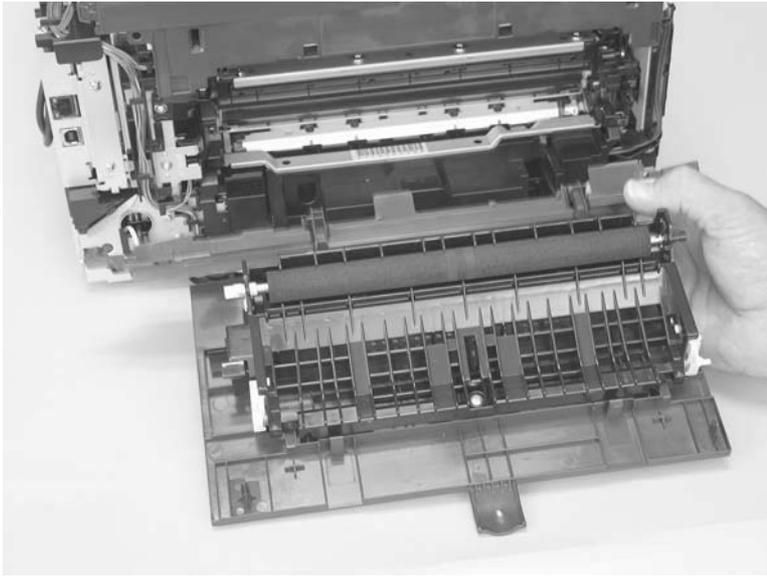
5. Carefully pry the rear-door hinge arms off of the hinge pins on the rear-lower cover to separate the rear cover (callout 3) from the rear door (callout 4).
