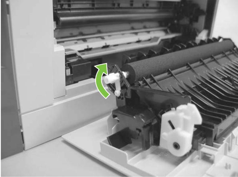
3. Remove the clip. Repeat these steps for the remaining retainer clip.
