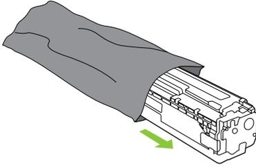
5. Remove the orange, plastic shield from the bottom of the new print cartridge.
