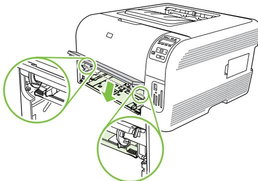
4. Remove the jammed sheet by pulling it straight out.
