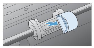
Position the new pickup roller in the slot. The circular and rectangular slots on each side prevents you from installing the roller incorrectly.
