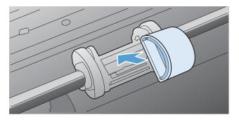
Rotate the top of the new pickup roller away from you until both sides snap into place.
