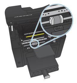
Release the small, white tabs on each side of the pickup roller, and rotate the pickup roller toward the front.
