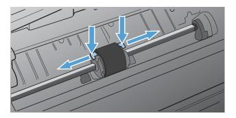
Gently pull the pickup roller up and out.
