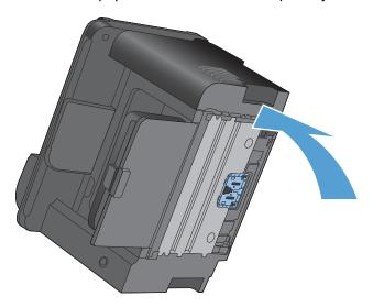
At the bottom of the product, unscrew the two screws holding the separation pad in place.
