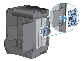
Insert the new separation pad, and screw it into place.
