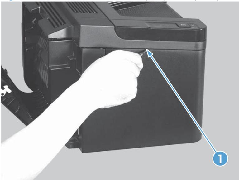
5. Rotate the back edge of the cover away from the product, and then remove the cover (callout 1).
