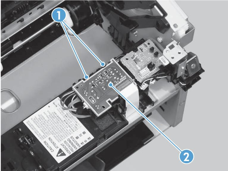
5. Release one tab (callout 1), and then remove the duplex-connector PCA (callout 2).
