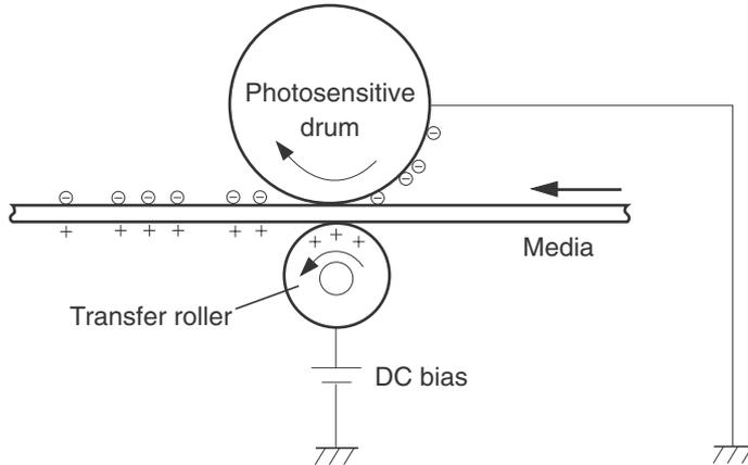
**Step 5:** The elasticity of the paper causes its separation from the photosensitive drum. A static charge eliminator aids separation by weakening any electrostatic adhesion.
