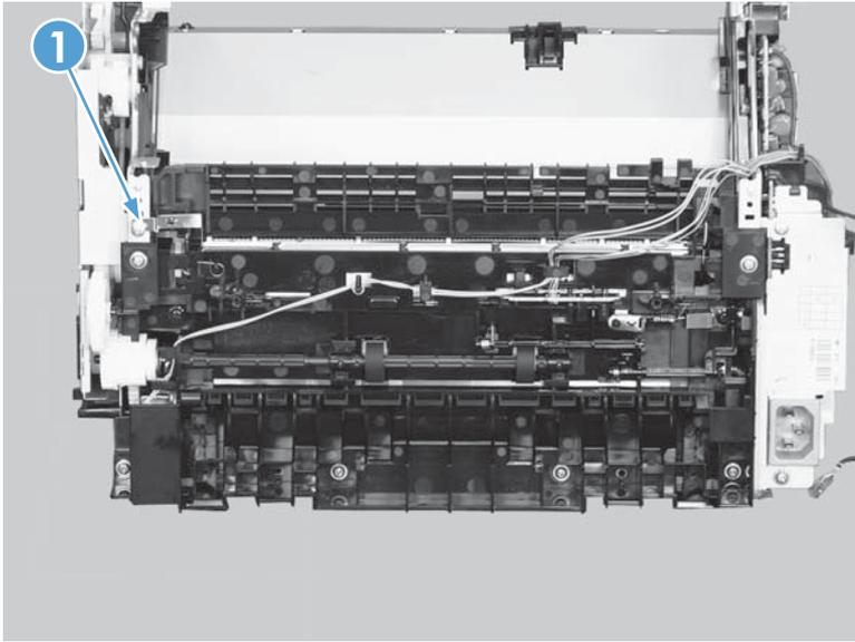
9. Remove six screws (callout 1), and then remove the pickup assembly (callout 2).
