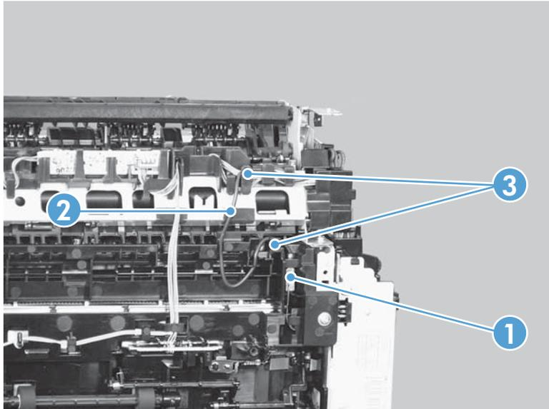
5. Disconnect four connectors (callout 1), and then remove the wire harnesses (callout 2) from the guide (callout 3).
