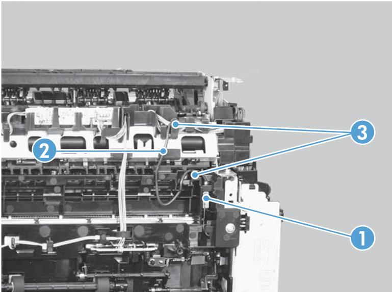
6. Disconnect three connectors (callout 1), and then remove the wire harness (callout 2) from the guide (callout 3).
