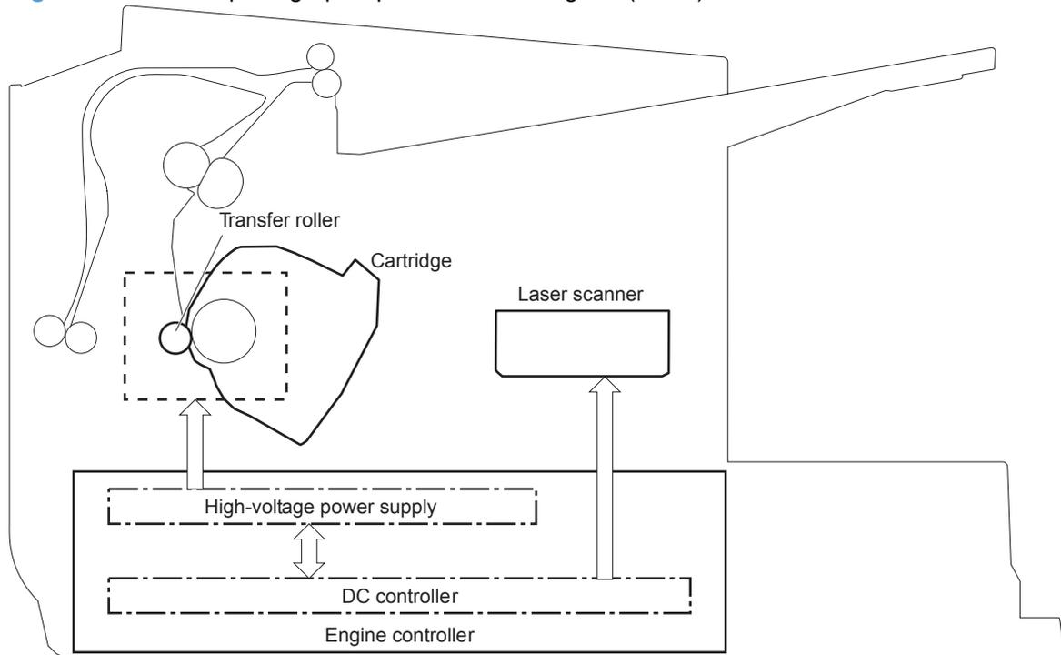
The DC controller rotates the main motor to drive the following components:
