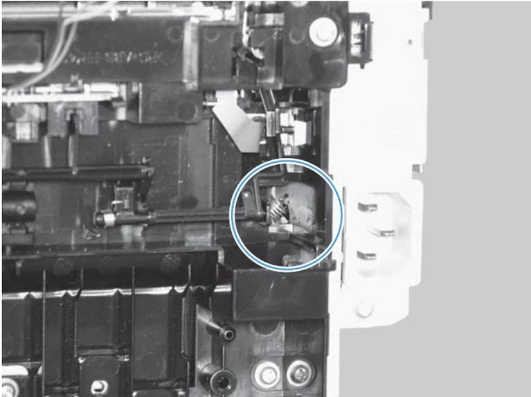
2. Push down the lift plate before installing the pickup assembly.
