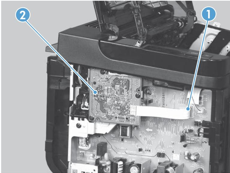
3. Remove three screws (callout 1), and then remove the formatter PCA.
