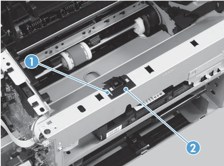
2. Remove four screws (callout 1), and then remove the scanner cover (callout 2) and the sheet-metal plate (callout 3) together.
