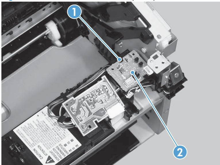
6. Disconnect two connectors (callout 1) and carefully set the PCA out of the way.
