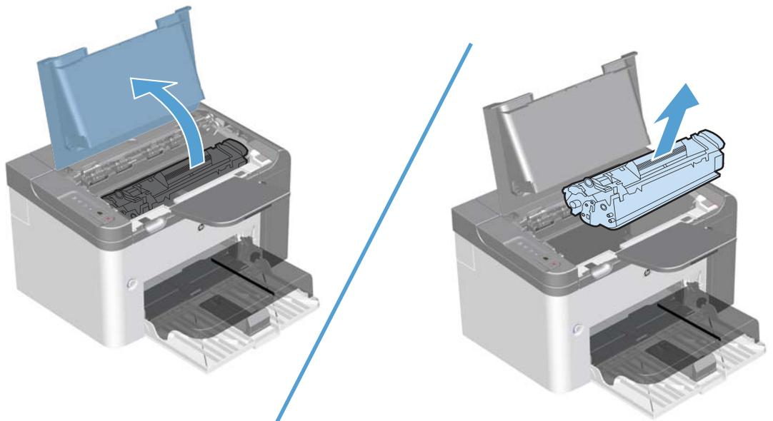
△ **CAUTION:** To prevent damage, do not expose the print cartridge to light. Cover it with a piece of paper.
