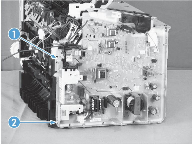
9. Remove three screws with washers (callout 1), and then remove the engine controller PCA (callout 2).
