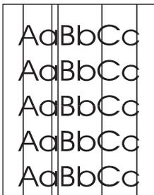
The photosensitive drum inside the print cartridge has probably been scratched. Install a new genuine HP print cartridge.
