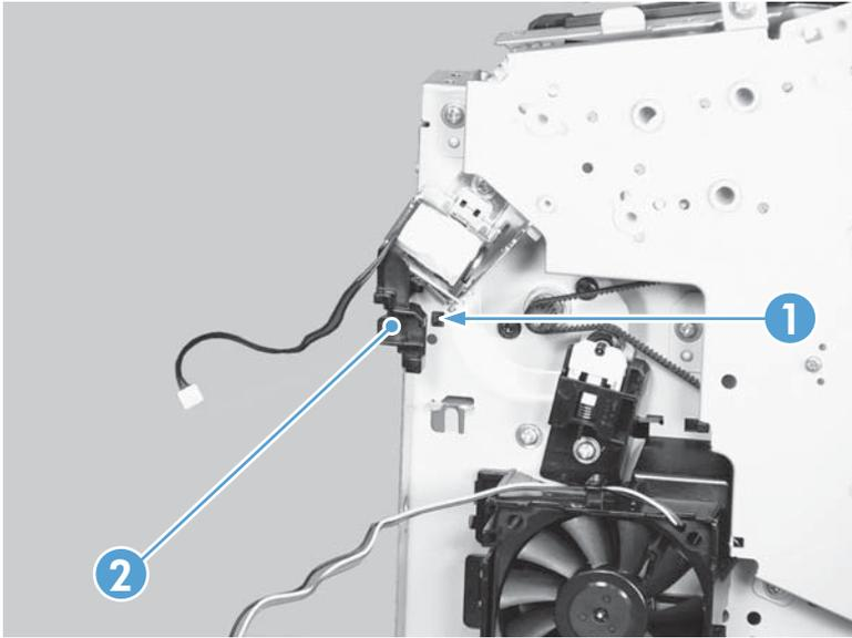
5. Remove one screw (callout 1), and then remove the duplex-reverse solenoid (callout 2).
