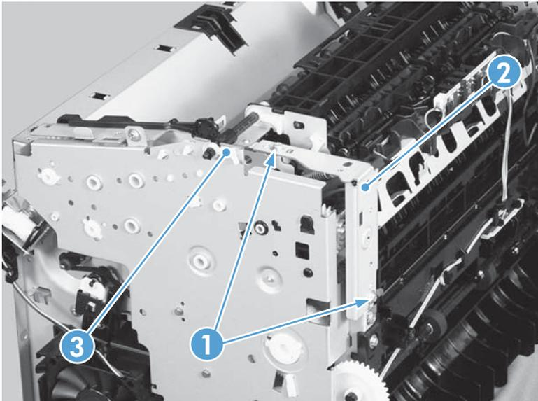
10. Remove three screws (callout 1) and then remove the fuser (callout 2).
