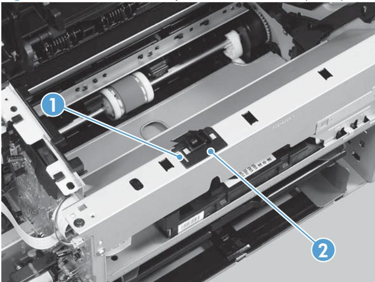
2. Remove four screws (callout 1), the scanner cover (callout 2) and the sheet-metal plate (callout 3).
