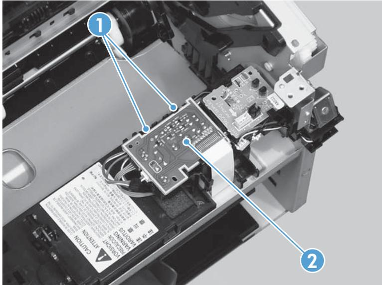
5. **Duplex models only:** Release one tab (callout 1), and then remove the duplex-connector PCA (callout 2).
