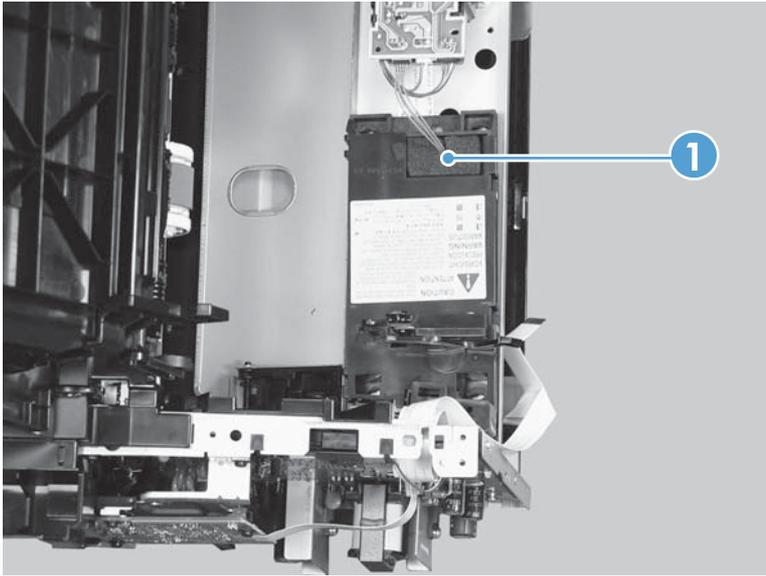
5. Disconnect one connector (callout 1), and then remove the laser/scanner assembly (callout 2).
