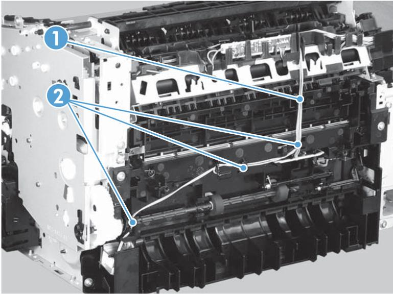
7. Remove one screw (callout 1), and then remove the pickup solenoid (callout 2).
