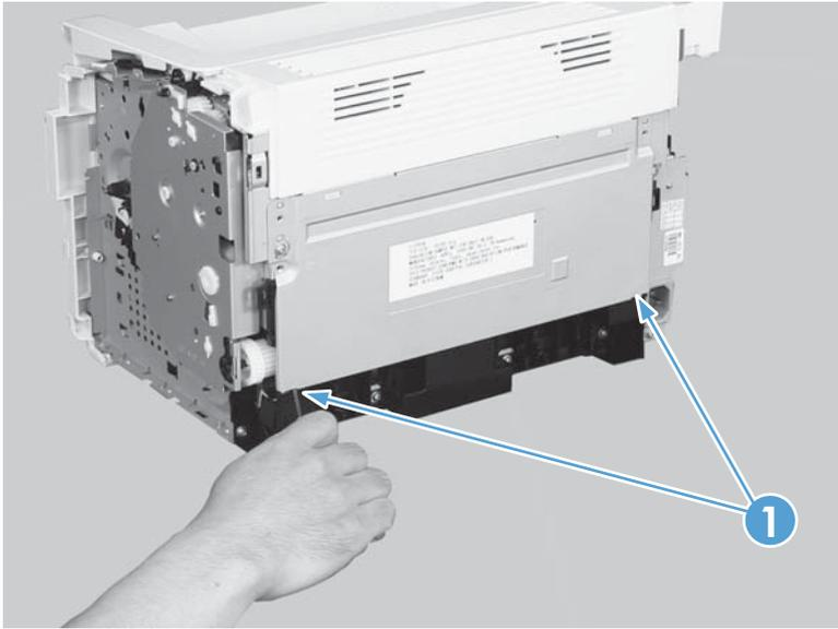
3. Rotate the bottom of the rear cover (callout 1) away from the product to remove it.
