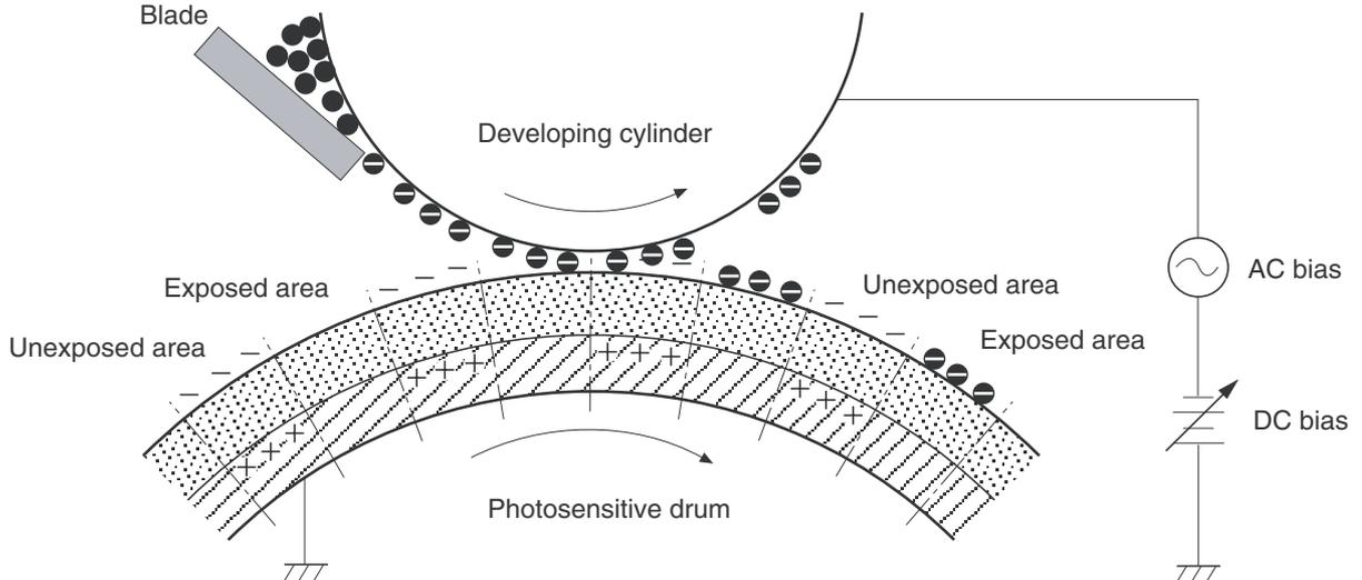
Toner acquires a negative charge from the friction that occurs when the developing roller rotates against the developing blade. The developing bias is applied to the developing roller to make a potential difference between the developing roller and the photosensitive drum. The negatively charged toner is attracted to the latent image on the photosensitive drum because the drum surface has a higher potential.
