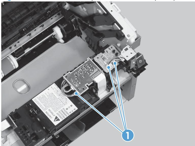
4. Release two tabs (callout 1), and then slightly separate the motor driver PCA (callout 2) from the product.
