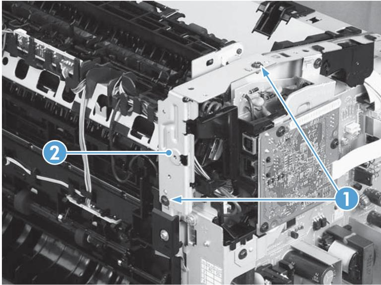
3. Remove one FFC (callout 1), remove three screws (callout 2), and then remove the formatter (callout 3).
