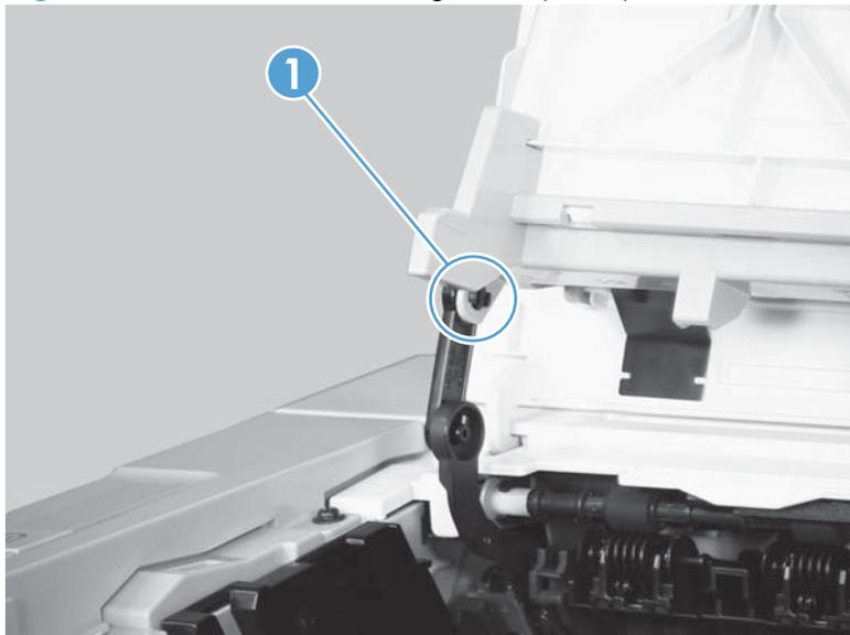
3. Release two pins (callout 1), and then remove the cartridge door (callout 2).
