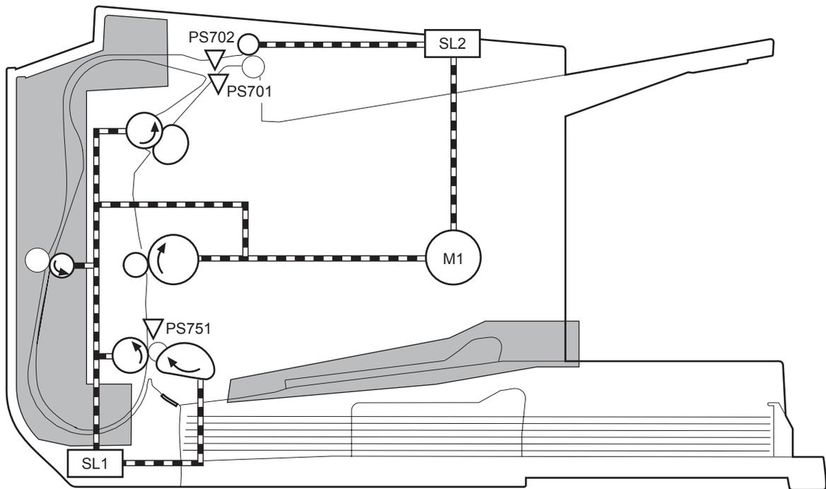
**Table 1-8** Photo sensors, motor, and solenoid
