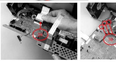
c.) Tilt the top of the ECU away from the printer and disconnect one ribbon cable (callout 29). Lay the ECU pan down on the work surface and remove three cables (callout 30). Remove ECU.
