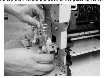
our name, an 7. Removing Fixing Drive Side Plate Assembly a.) Release three gear tabs (callout 39) and remove gears.
