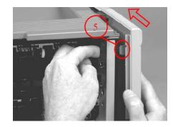
d.) Remove Left Cover by removing two screws (callout 4), then open toner cartridge door. Release one tab (callout 5) the back of printer by pressing the tab through a hole in the chassis, then pull cover at the back slightly. Slide the cover toward the front to printer to clear the tabs at the front and then lift cover away from the printer
