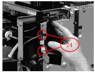
**5.** Remove **ECU** a.) Remove the air duct by squeezing the two release tabs (callout 24) and lift off printer.
