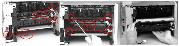
b.) Disconnect two cables from the right side of the fuser cavity (callout 21). Remove one cable from below the power cord inlet (callout 22). Remove four screws (callout 23). Slide fuser out the back of the printer.
