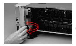
c.) Remove **I/O cover** by rotating the cover t clear tabs at the right side of the printer.
