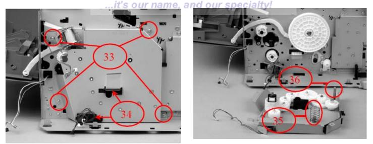
b.) Remove four screws (callout 33) from the gear assembly plate. When removing the gear plate from the printer, be care full when pulling the cables through the gear plate (callout 34).
