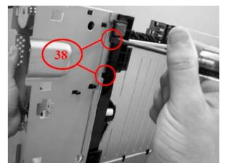
c.) Remove the power switch guide (callout 37) by using a flat blade screwdriver to release two tabs (callout 38).
