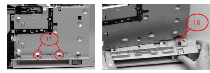
b.) Remove **Right Side Handle** by removing two screws (callout 17). Slide the handle toward the back of the printer until the power switch (callout 18) is adjacent to the hole in the printer chassis then rotate the handle so that the power switch clears the hole. Remove handle.
