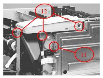
h.) Remove **Control Panel** by disconnecting one cable (callout 11), then remove three screws (callout 12). Lift control panel off printer.
