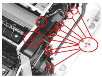
Disconnect nine cables (callout 25); six cables at the top of the ECU and three cables at the front of the ECU. Remove the cartridge door switch (callout 26) from its mount.
