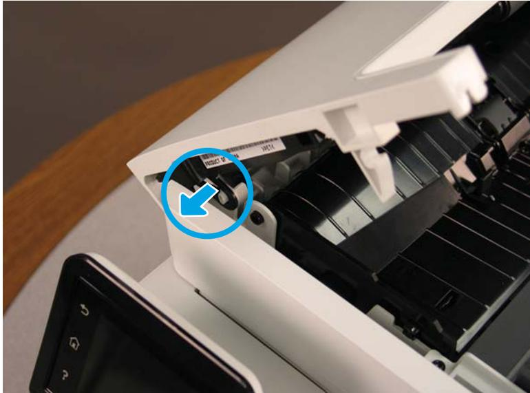
3. Carefully insert a small, flat-blade screwdriver between the separation pad support and the document feeder case. Rotate the end of the screwdriver towards the separation pad to release the support.
