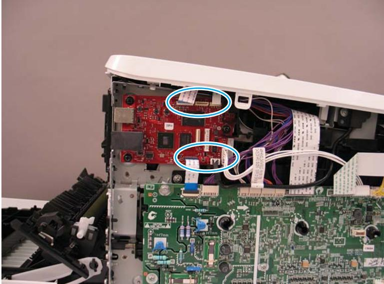
2. Remove three screws (callout 1), and then remove the PCA from the printer.
