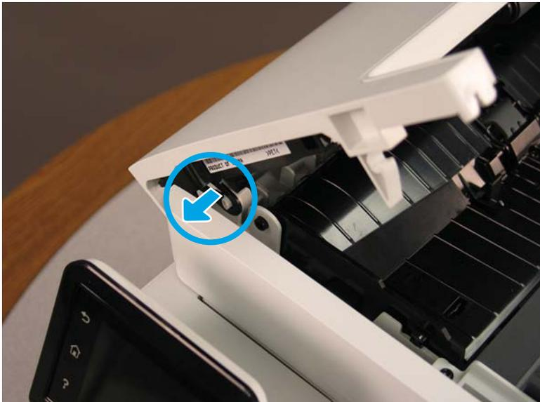
3. At the front of the printer, use a small, flat-blade screwdriver to flex the inner cover away from the outer cover (callout 1), and then lift up to release the arm from the hinge pin (callout 2).
