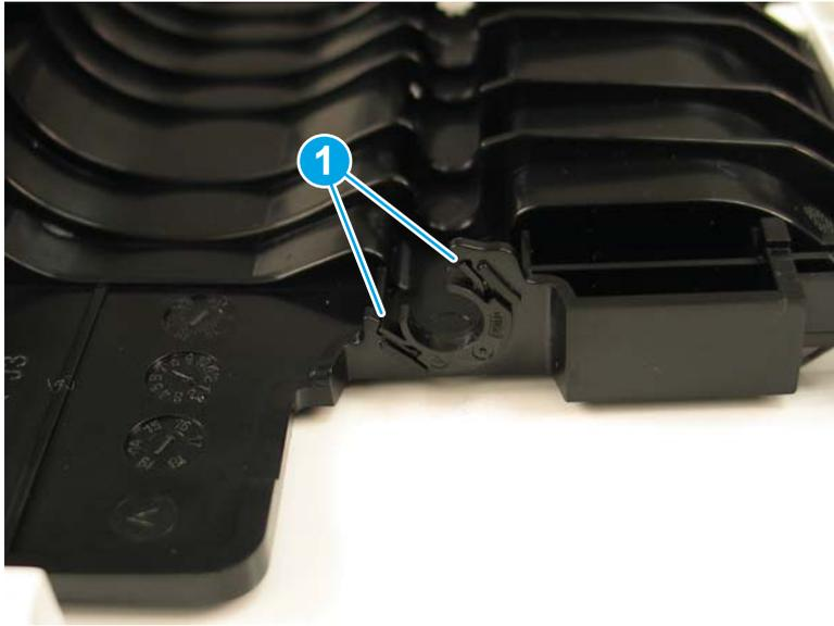
3. Remove the bearing from the top cover.
