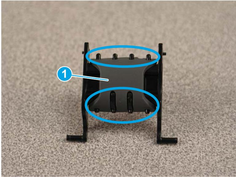
6. To remove the separation pad spring, turn the separation pad support over, and then remove the spring (callout 1).
