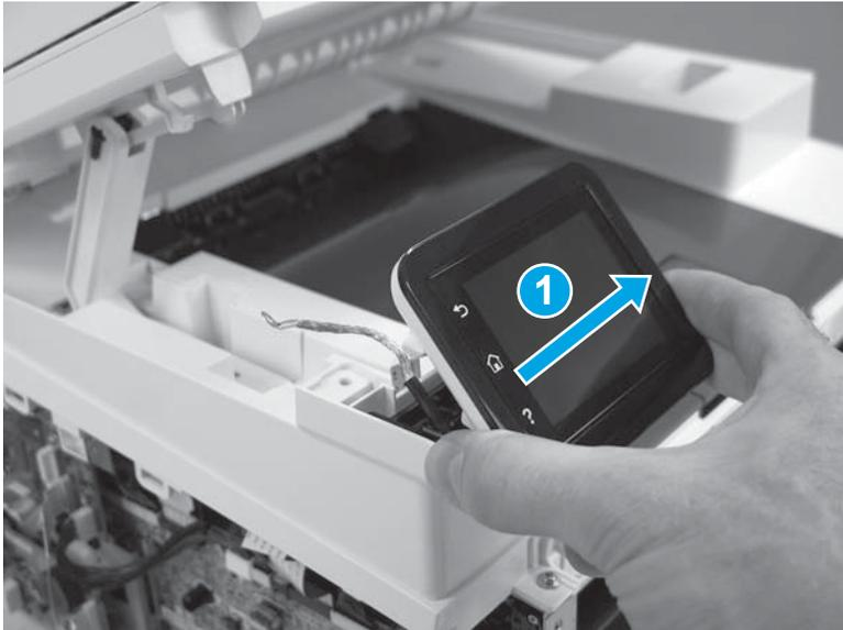
6. Rotate the control panel forward to release it (callout 1), and then lift it slightly away from the printer.
