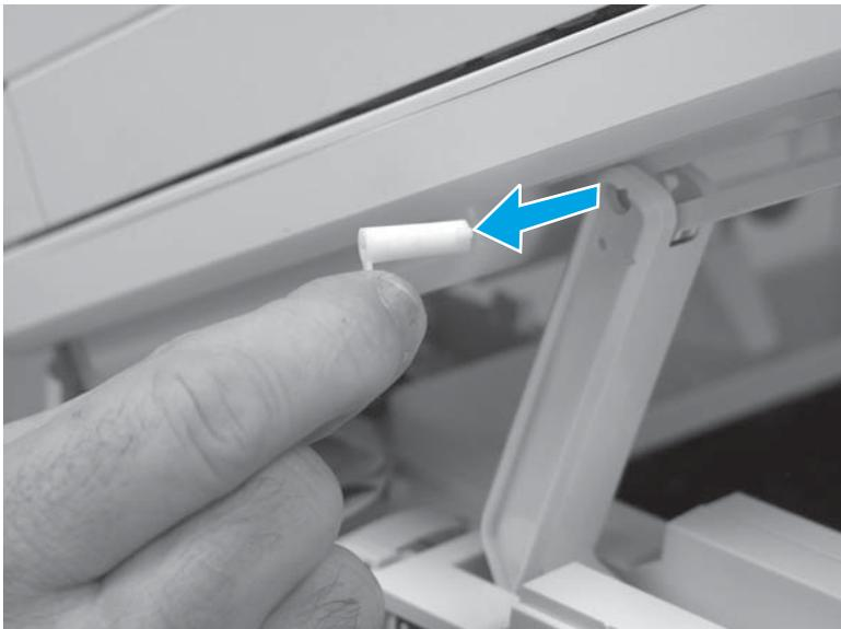
4. Rotate the hinge arm down.
