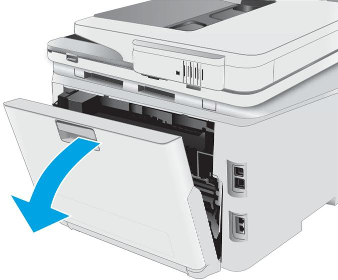
Step 2: Remove the duplexer door assembly
