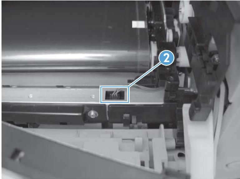
5. Carefully lift up on the front of the ITB to release it.
