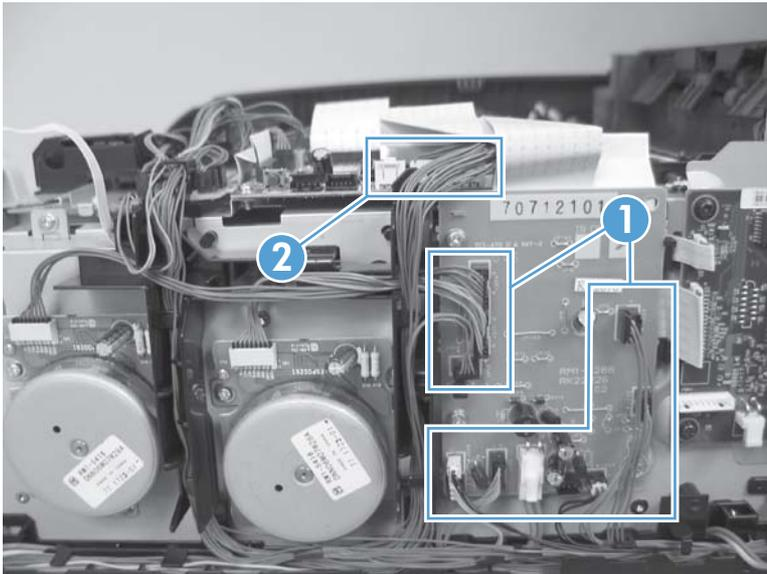
2. Remove three screws (callout 1), and then remove the intermediate PCA.
