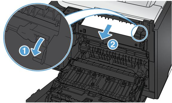
3. If necessary, remove any visible paper from bottom side of the duplexing unit.
