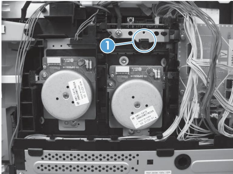
5. Rotate the top of the retainer away from the chassis, and then lift it up to remove it.
