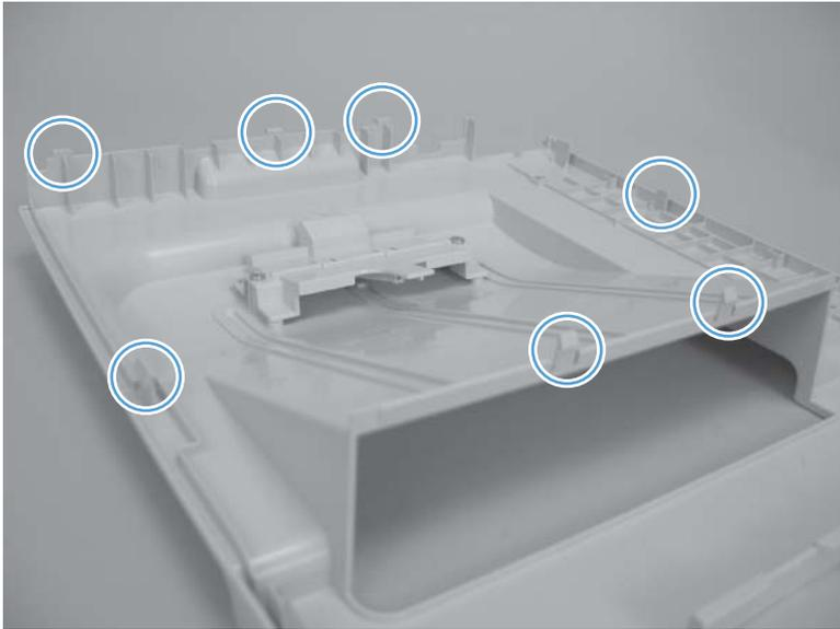
5. Carefully rotate the back side of the top cover up and off of the product to release the tabs, and then remove the cover.
