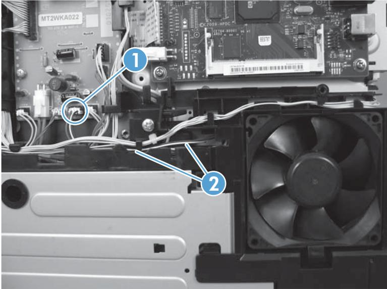
3. Release one tab (callout 1), push down on the fan to release it from the mounting points (callout 2), and then remove the fan.
