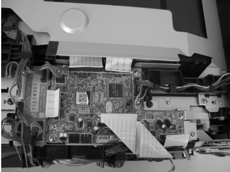
2. Remove four screws (callout 1) and then remove the DC controller PCA.
