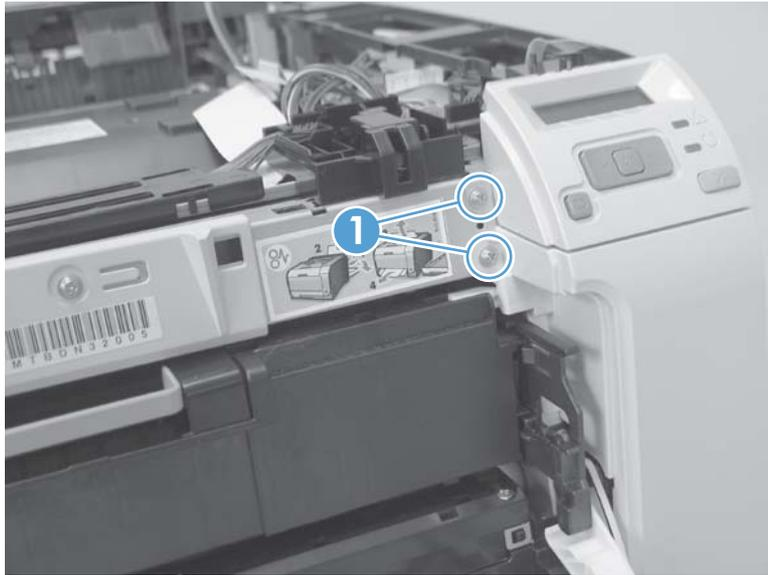
3. Remove the control-panel assembly.
