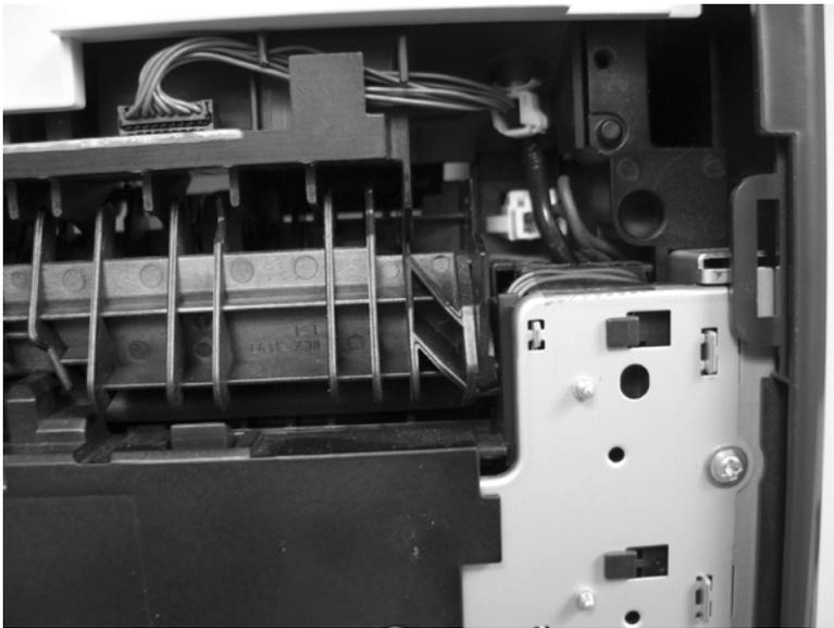
5. Carefully release a feed-guide hinge pin from the rear cover to release the feed guide.
