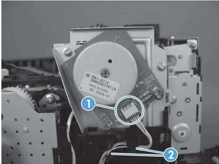
3. Remove three screws (callout 1), and then remove the fuser motor assembly.
