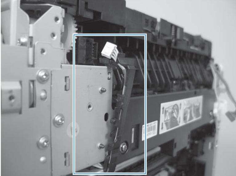
5. Carefully disconnect one connector and rotate the connector and the top portion of the guide away from the fuser (callout 1).
