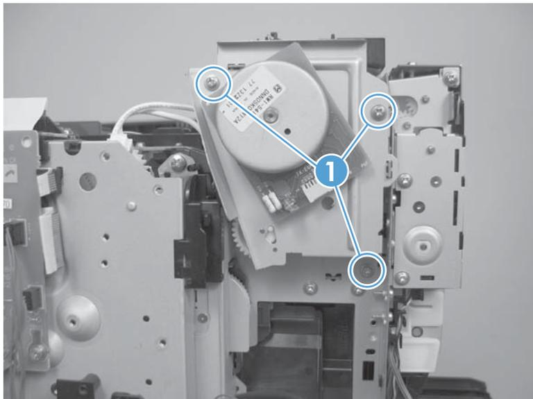
4. Be careful, the spring and the gears behind the fuser motor assembly are not captive.
