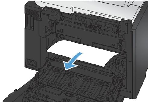
4. If you can not see any jammed paper, lift the duplexing unit using the tab on the side of the duplexing unit.
