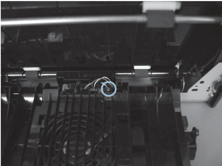
2. Slide the assembly toward the power cord side of the product to release the hinge pin.
