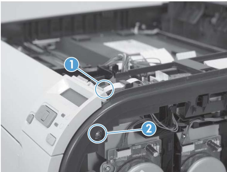
2. Open the front door, and then remove two screws (callout 1).
