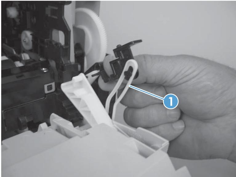
6. Support the door assembly, and carefully release the pin on the right-side link.
