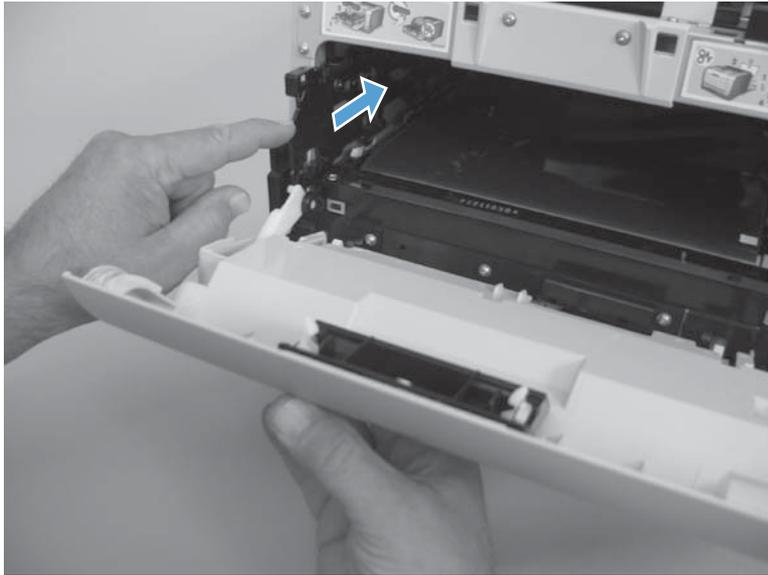
9. Support the door assembly, and carefully release the lower pin on the left-side link.
