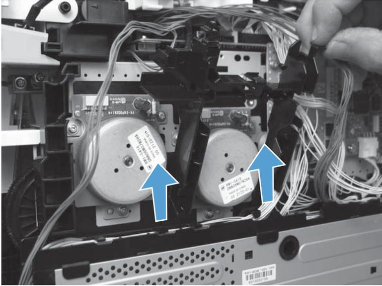
6. Remove three screws (callout 1) to remove motor M1, or remove three screws (callout 2) to remove motor M2.
