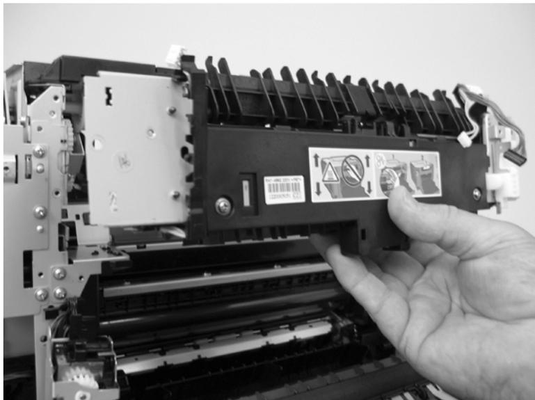
8. **Duplex models only:** Remove two screws (callout 1) and remove the duplex-gear assembly (callout 2). Install the assembly on the replacement fuser.
