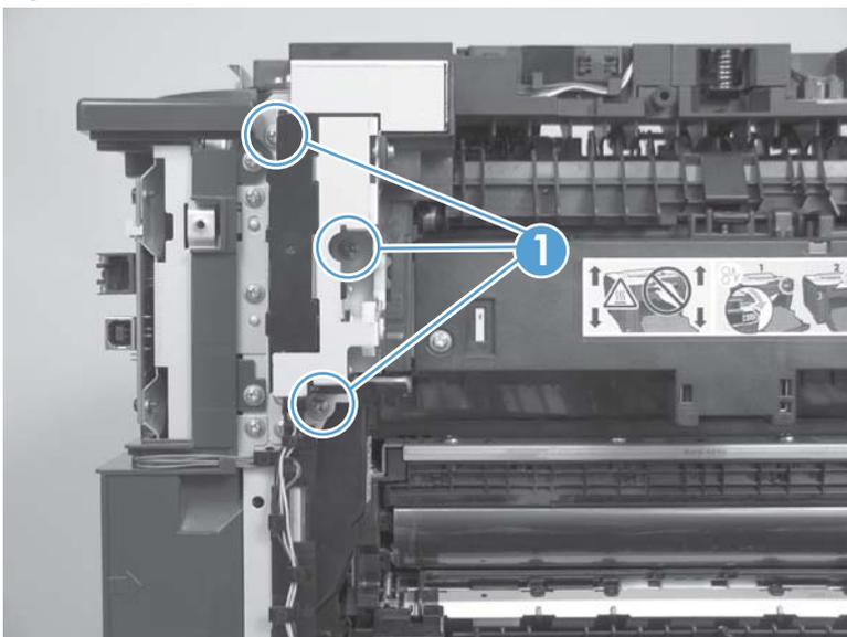
2. Disconnect two connectors (callout 1), and then release the wire harnesses from the guide (callout 2).
