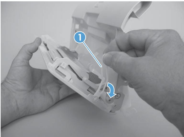
2. Remove the retainer arm from the door assembly, and then install it on the replacement-door assembly.
