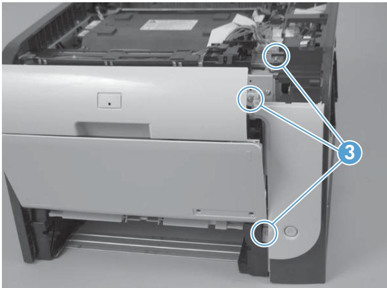
4. Disconnect two connectors (callout 1), release the fan wire harness from the guide (callout 2), and then remove three screws (callout 3).
