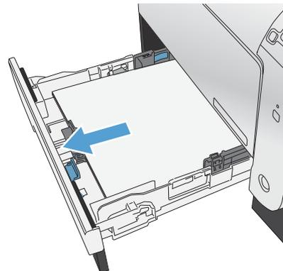
2. Remove the jammed sheet by pulling it straight out.
