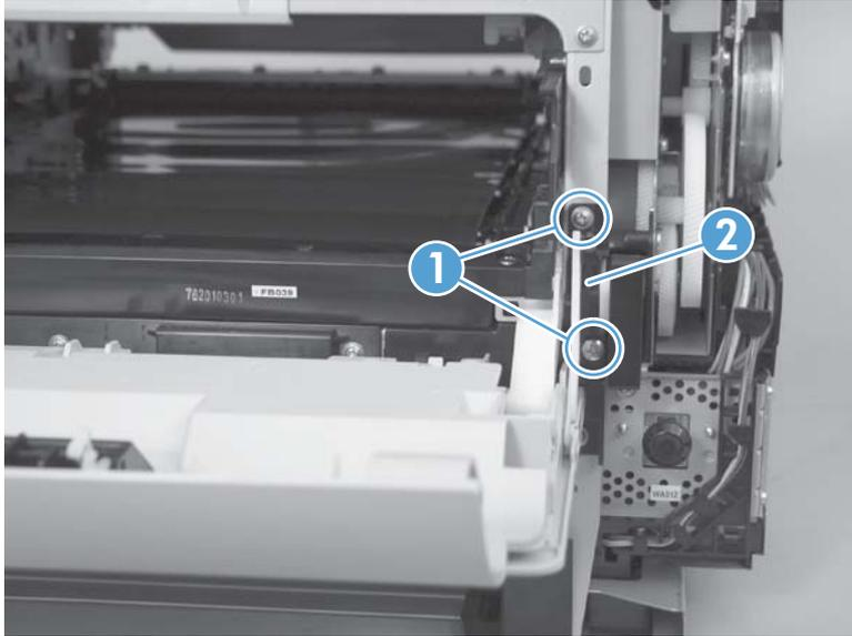
5. Release the bushing from the door-retainer link (callout 1).
