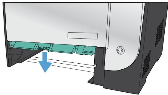
4. Remove the jammed sheet by pulling it straight out.
