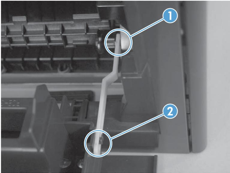
**Figure 1-53** Replace the link guide (duplex products)
