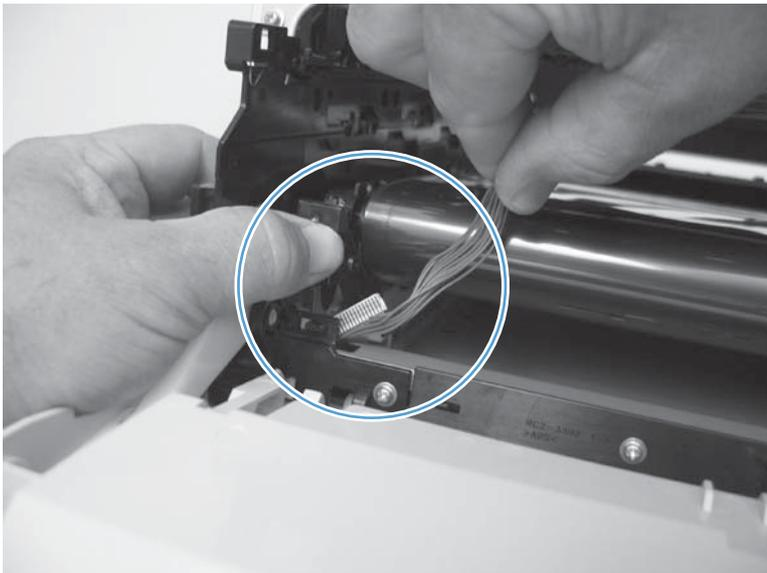
2. Use a small flat blade screwdriver to guide the connector through the hole.
