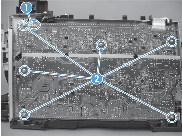
5. Release ten tabs (callout 1), and then remove the high-voltage power-supply PCA.
