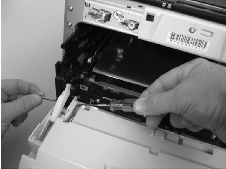
3. Use a precision-point screwdriver to push the right-side door pin out of the link.
