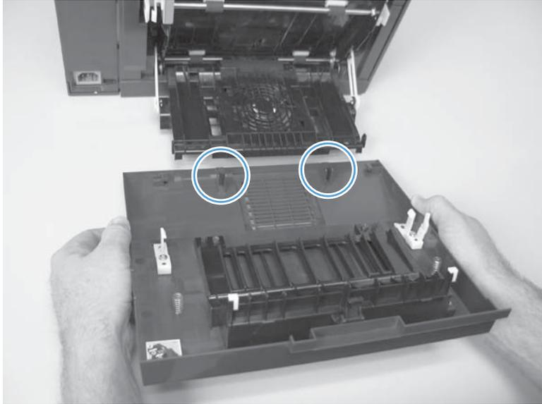
5. Slide the door away from the product to release two tabs, and then remove the door.
