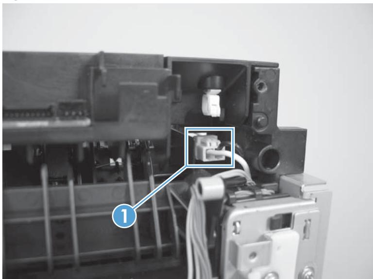
4. *Before you proceed*, look at [Figure 1-136 Remove the fuser \(4 of 8\) on page 94](#). In the following step, the connector and guide will be separated from the fuser. You **must not** use too much force and damage the lower portion of the guide. If the guide is damaged, the fuser must be replaced.
