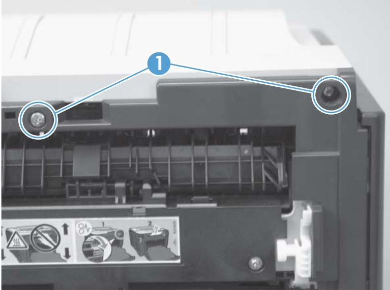
3. Slightly separate the cover from the product, and rotate the cover down and then away from the product to remove it.
