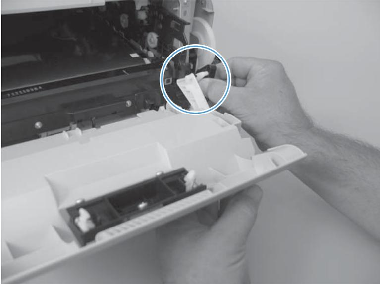
7. Support the door assembly, and carefully release the upper pin on the left-side link.
