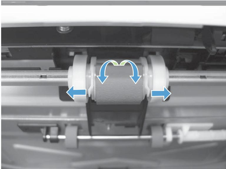
5. Release the retainer tabs, and then remove the separation pad from the base.
