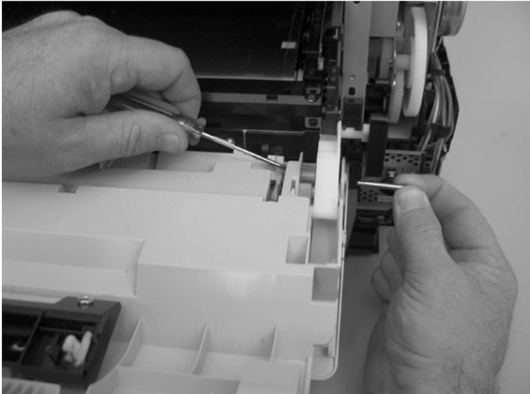
4. Remove two screws (callout 1) and separate the door bushing (callout 2) from the chassis.
