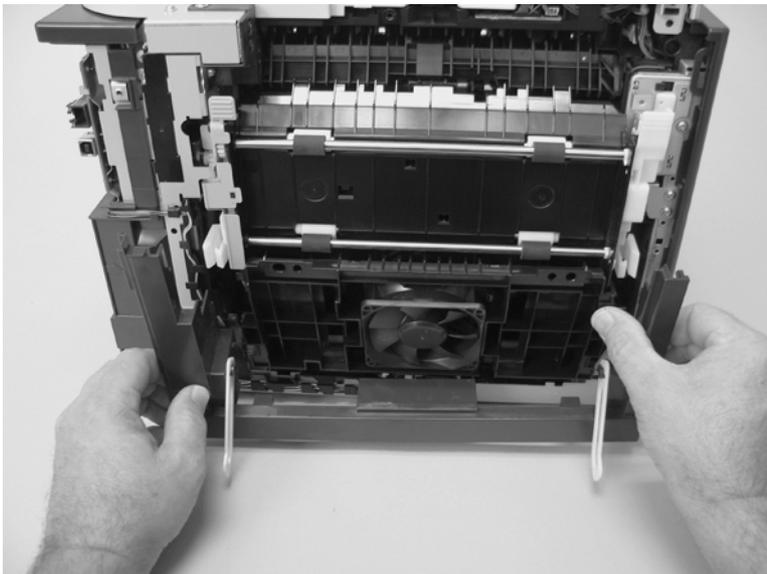
6. Rotate the rear-door link until the slot in the link aligns with the tap on the link-hinge pin, and then remove the rear-door link. Repeat this step for the remaining rear-door link.
