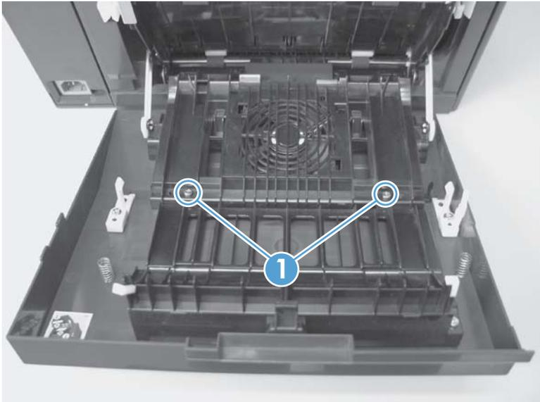
4. Before you remove the rear door, take note of the mounting tabs on the door.
