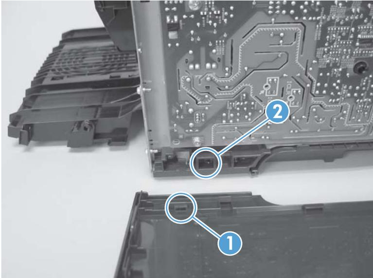
2. When you reinstall the left cover, ensure that the pin on the cover (callout 1) aligns with the slot (callout 2) in the product.
