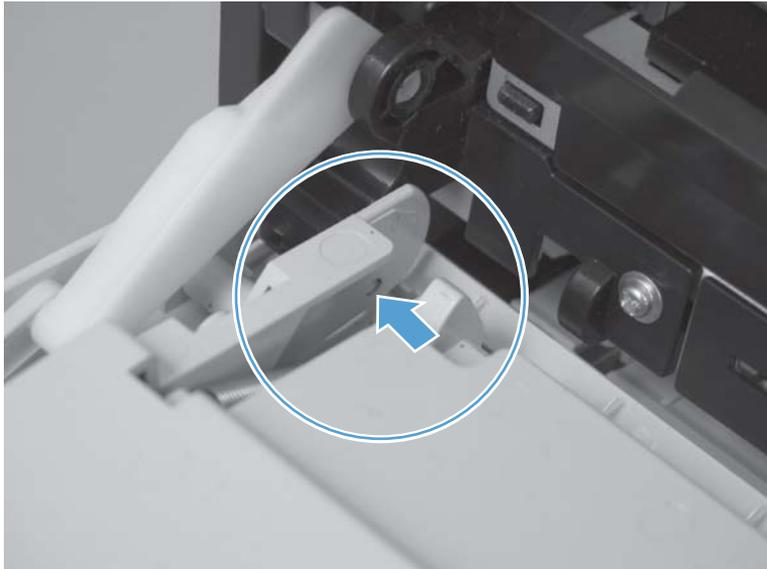
2. Use a precision point screwdriver to push the left-side door pin out of the link.
