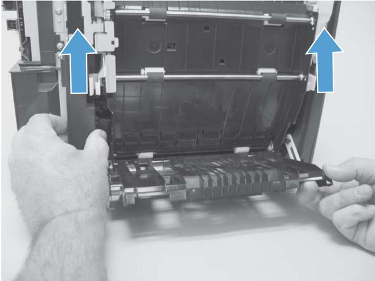
5. Slightly lift up the rear-door rib assembly, and then carefully slide the cover away from the product to remove it.
