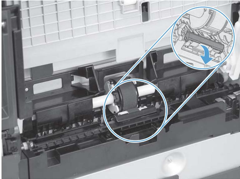
3. Release the roller holder to release the roller-locking pins. Remove the separation roller.
