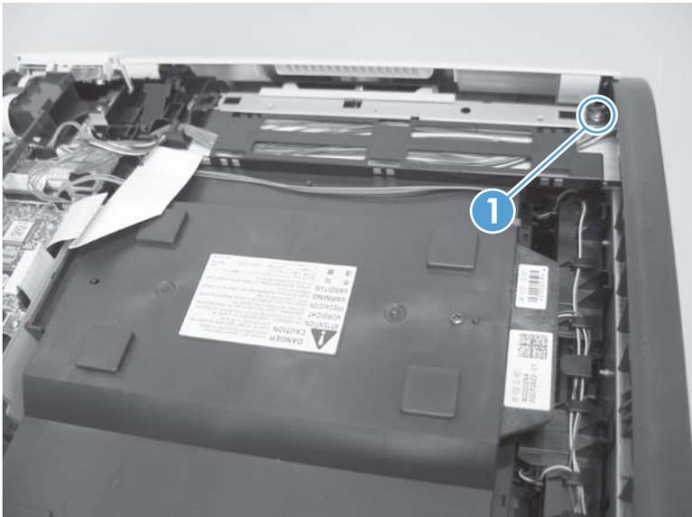
2. Slightly lift up on the cover, and then rotate the top of the cover away from the product.
