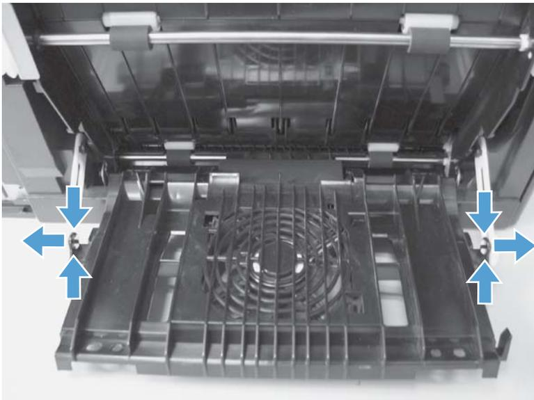
2. Open the duplex-feed assembly, release one tab (callout 1), and then slightly separate the cover from the product.
