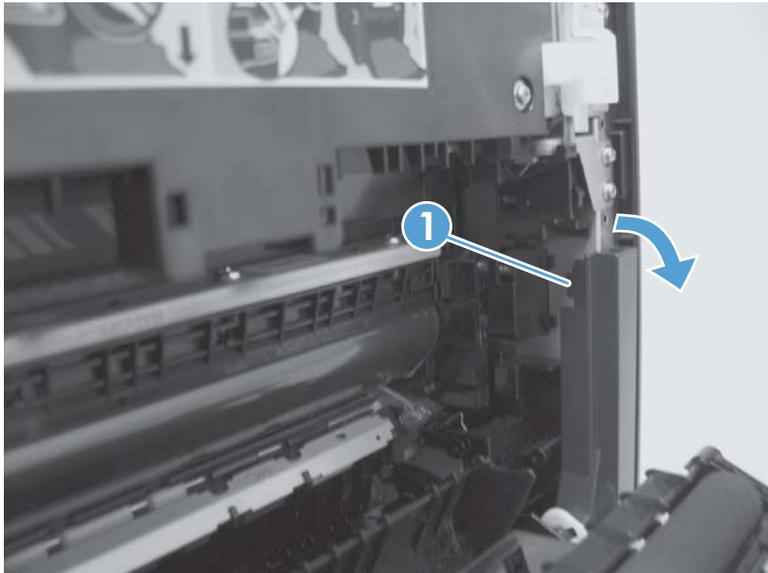
4. Close the duplex assembly, lift up on one side of the cover, and then lift up the other side of the cover to release it.
