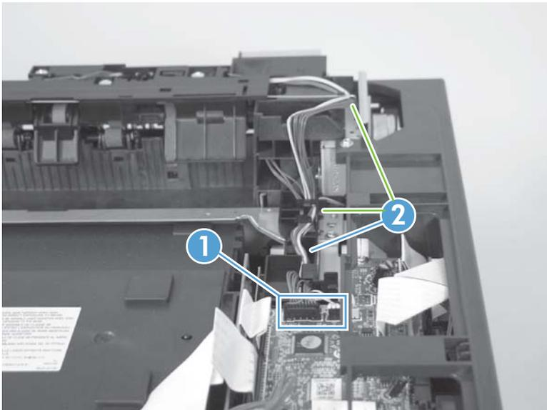
2. Disconnect two connectors (callout 1), and then release the wire harnesses from the wire clip (callout 2).
